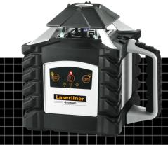
The Quadrum M350 S is a fully automatic rotary laser for the exact alignment of horizontals and verticals. With a radius of 350 metres, the laser reception range is extremely large. The functions can easily be controlled with the remote control up to a max. distance of 40 metres. The manual tilt mode allows gradients to be created. In the event of external influences, an
