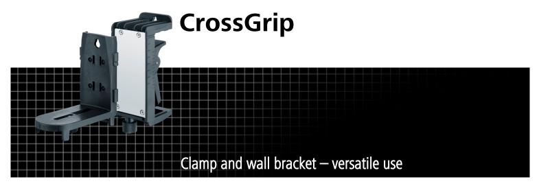
This magnetic clamp and wall bracket is suitable for all laser measuring devices with 1/4" thread. It has eyelets for direct mounting on the wall. Strong adhesive magnets on the back enable attachment to metallic surfaces. Horizontal or vertical mounting on drywall construction profiles is possible by means of clamping brackets. By adjusting the set screw, the opening width of the clamp can be regulated.
