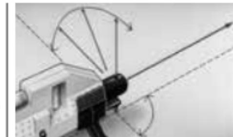
The 90° beam splitter allows the laser beam to be additionally deflected by 90°.
